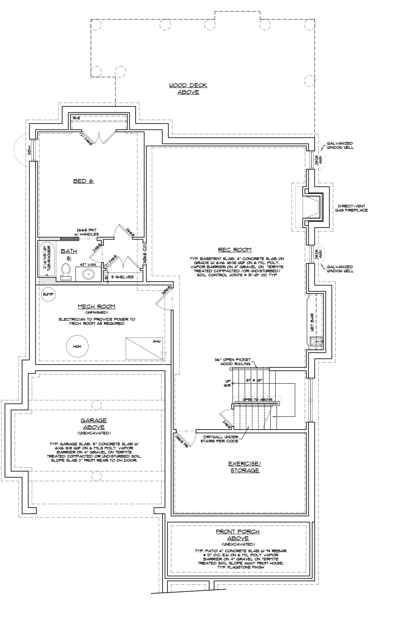
NOTE: ALIGN TOPS OF WINDOWS, BULKHEADS AND CASED OPENINGS TO R.O. OF INTERIOR DOORS, U.O.N.
